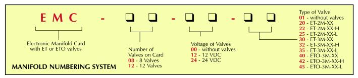
EMC-08-00-01 and EMC-12-00-01 are part numbers for cards without any valves, and without manifold. Manifold mounting hardware is included. Manifolds may be ordered separately, if desired. Part numbers are: 15482-8 and 15482-12.
